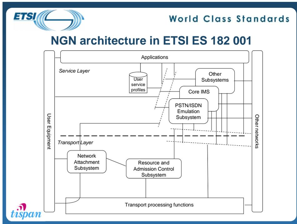
Figure 3-3. Illustration of the ETSI TISPAN NGN architecture.
