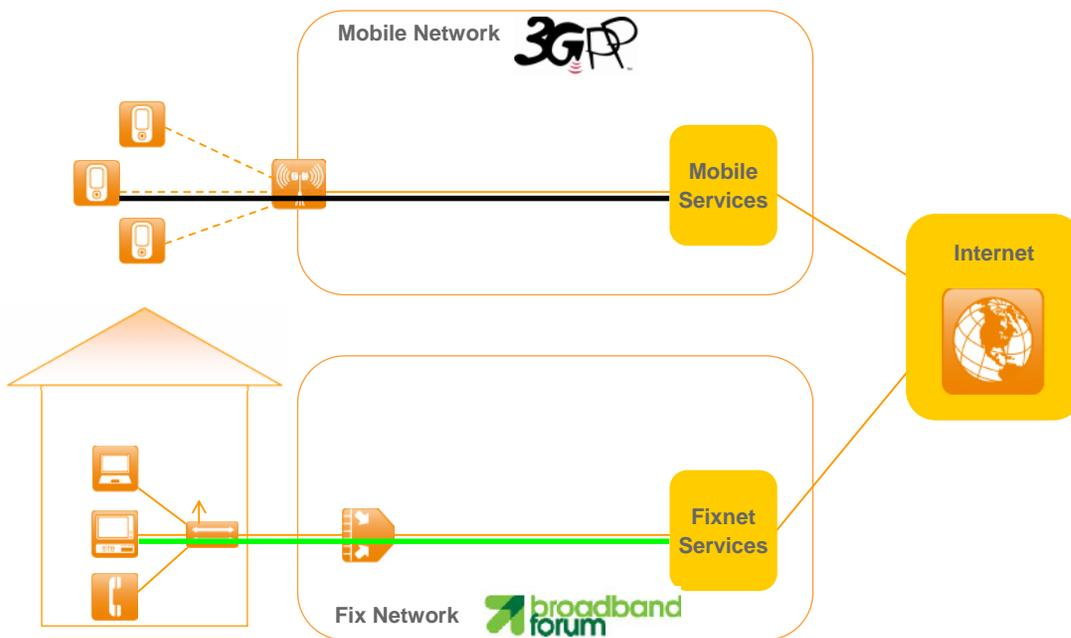
**Figure 2-2. Separated fix networks and mobile networks**
