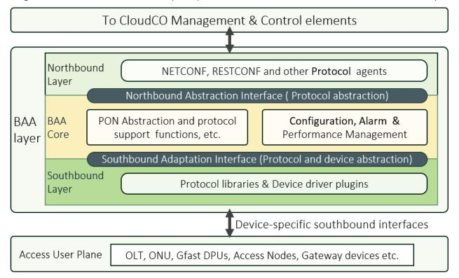
**Abstraction** has been a fundamental concept of layered telecommunications architectures for decades. It fosters independent solutions for devices, compute and network elements, security and software to coexist. The layered architecture shows how the BAA layer enables independence of the north and
