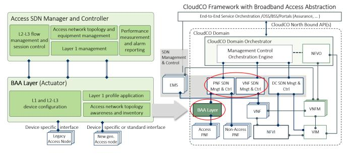
The SDN Managers & Controllers are responsible for Fault, Configuration, Accounting, Performance, Security and Flow Control management functionalities for Cloud CO Network Functions. They implement the Management & Control Plane that governs the overall user plane represented by the service graphs that chain PNFs, VNFs and networking resources together within the CloudCO Domain.
